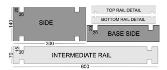
Notches are started 25mm in from the end of the timber and are 20mm wide and 20mm deep for the side pieces and 20mm wide and 15mm deep for the cross rails. If you are using a different thickness timber you will have to adjust these measurements.
