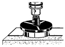
If using a hole saw, buy the best ones you can afford. Cheap saws overheat quickly and lose their edge even quicker.
