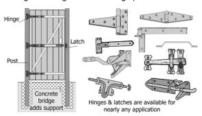
Now you can fit the gate latch. The positioning of the latch will depend on the height of the gate. For gates that cannot be reached over, a ring gate latch is a good choice, alternatively you cut a hole in the gate big enough to put a hand through to access the latch. Gates of a lower height can be reached over so the normal type of latch would be an auto gate latch.
